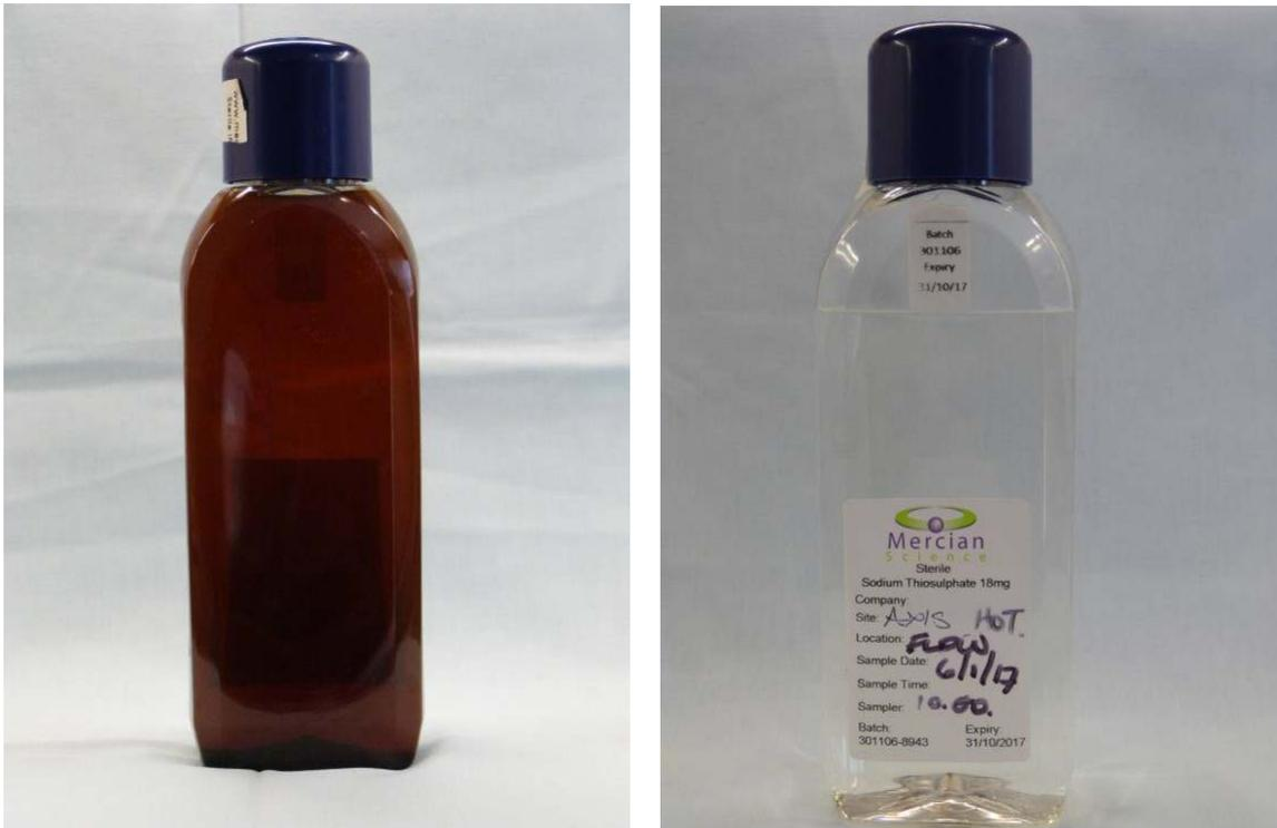
**Fig. 2: Water samples taken from a 50,000 litre system in a 6-storey building in Gateshead (before and after Oxypod installation).**
